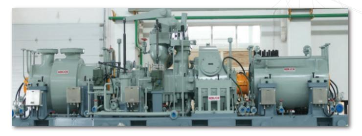
The Steam turbine, as the driver, was also designed and manufactured in NEW JCM works in accordance with API 612, 6th Edition Standard. Based on KELLOGG requirements to meet the heat and material balance, the selected turbine was an extraction condensing type.
