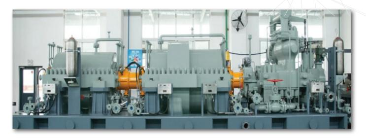
The Steam Turbine, as the driver, was also designed and manufactured in NEW JCM works in accordance with API 612, 6th Edition Standard. Based on KELLOGG requirements to meet heat and material balance the selected turbine was a back pressure type.
