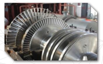
The Steam turbine, as the driver, was also designed and manufactured in NEW JCM works in accordance with the API 612, 6th Edition Standard. Based on KELLOGG requirements to meet the heat and material balance, the selected turbine was an induction condensing type.
