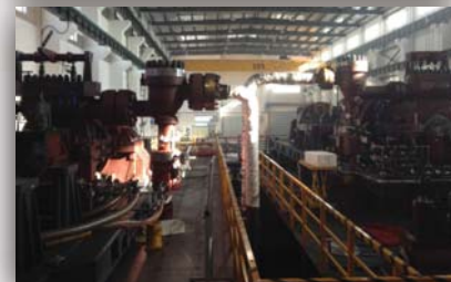
Process Air Compressors (LP/HP) c/w Mechanical Drive Steam Turbine (Mechanical Running API617 and String Tests)
