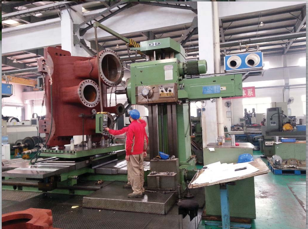
Compressor Casing Machining
