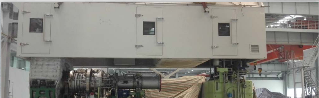
Complete Gas Turbine Packaging c/w Gas Turbine Core Engines Oil Lubrication package and Sound Enclosure
