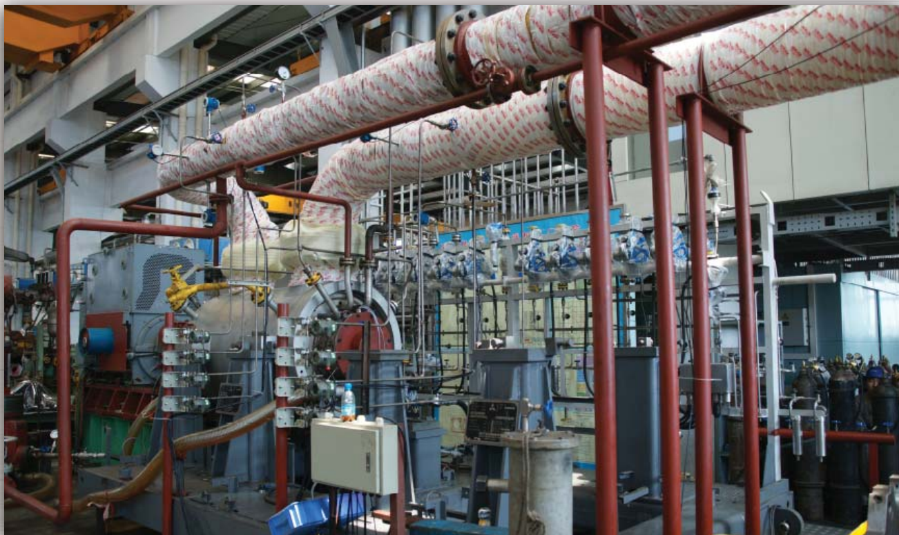
Pakistan national oil and gas companies Natural Gas Compressor : ASME PTC10-2 performance test With Approved test protocol by SGS France.
